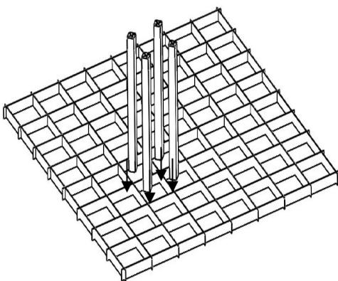
Line up and insert the wood rack pieces into the metal frame. Use a rubber mallet to install into the metal cross frame. Repeat until all wood rack pieces are installed.
