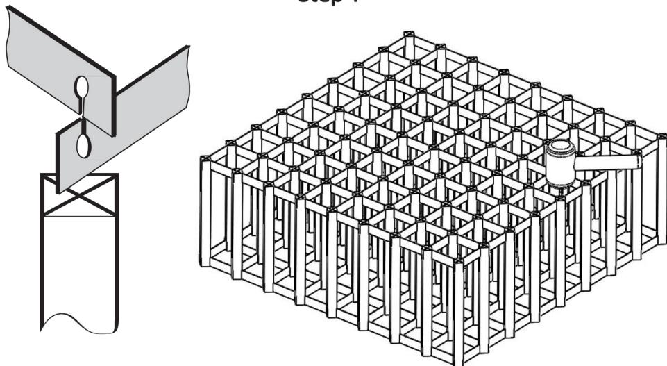
Insert the second section of the metal frame into the first and using a rubber mallet complete the installation into the wood pieces.
