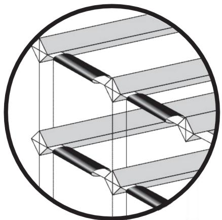
The bottle neck label protectors snap onto the front side of the metal frame as shown.
